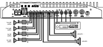
System 2 – The P850 is used in 8-channel mode. Channels 1/2 are high-passed for front tweeters. Channels 3/4 are band-passed for front midrange. Channels 5/6 are high-passed for rear speakers, and channels 7/8 are low-passed for subwoofers. Although shown as a 4-channel input, the source unit can be either 2- or 4-channel.
